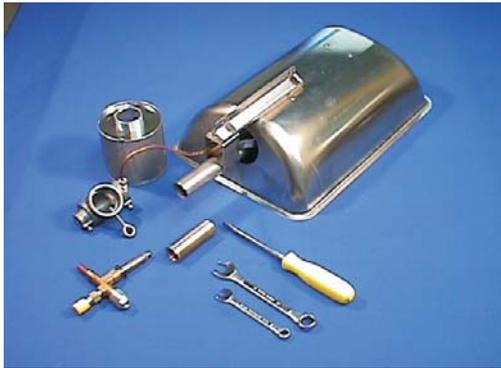
9. Remove brass venturi from burner pipe.
