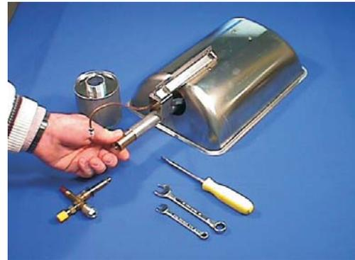
8. Locate brass venturi within the burner pipe.
