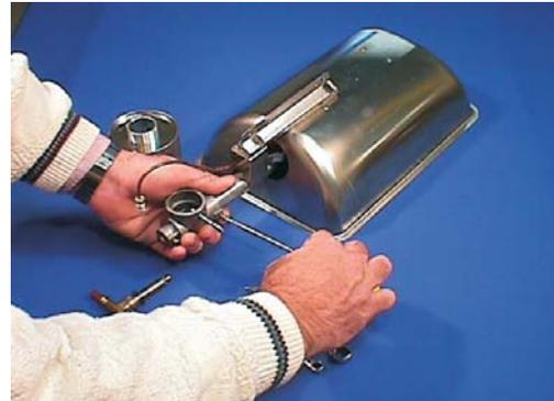
6. Loosen 2<sup>nd</sup> screw in the tee piece.
