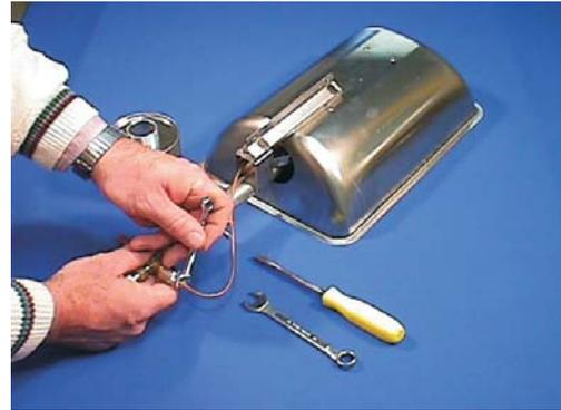
2. With a 5/16" or 8mm wrench, loosen thermocouple from safety device.
