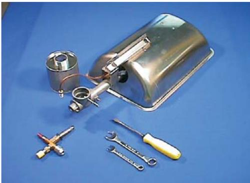
5. Remove the safety device/jet holder assembly from of the tee piece.
