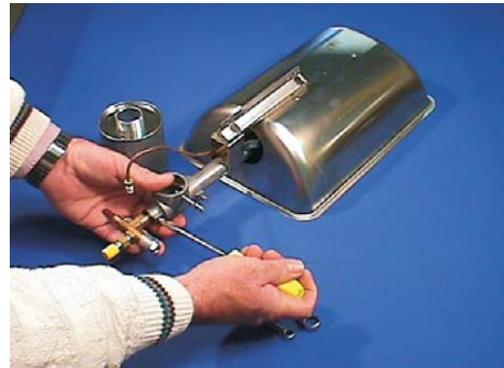
4. Loosen 1<sup>st</sup> screw in the tee-piece.
