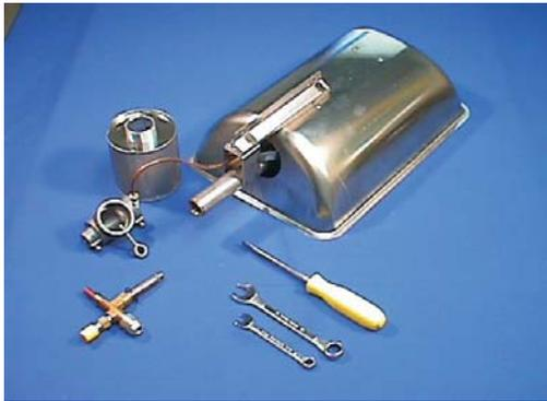
7. Remove tee piece from the burner pipe.
