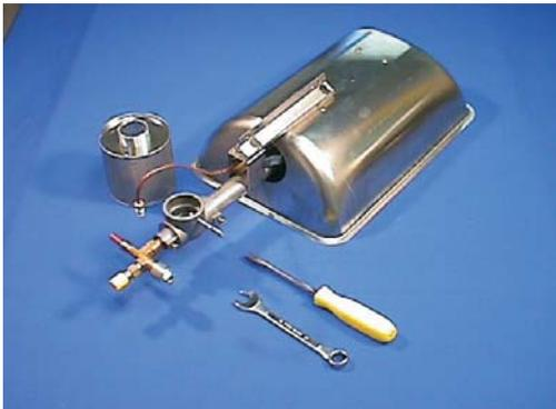
3. Rotate thermocouple out of your way.
