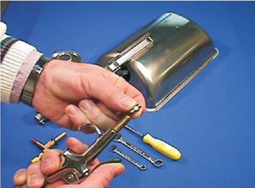
15. To clean the jet orifice apply compressed air to both ends of the jet.
