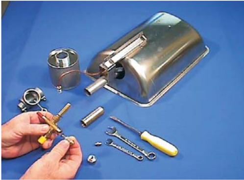
13. Remove interior coil from safety device.
