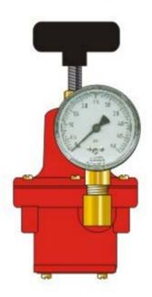
The PR-300/M 15kg gas regulator is used as a manual control or primary regulator with heaters operating between pressures of 0.1 – 4.5 (5-310 mbar) and 0.1-20 psi (5-1400 mbar) A pressure gauge is included. The PR-300/M will control up to 24 M8's or 50 M2's and will withstand direct tank pressure.
