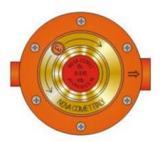
The PR-190 4kg gas regulator is used as a manual control or primary regulator with heaters operating between pressures of 50-190 mbar A numbered dial (1-10) represents the output pressure from minimum to maximum. The PR-190 is typically used to control Stype Gasolec heaters.
